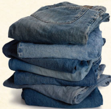
Acoustic insulation in interior walls is composed of recycled cotton—primarily old blue jeans.
